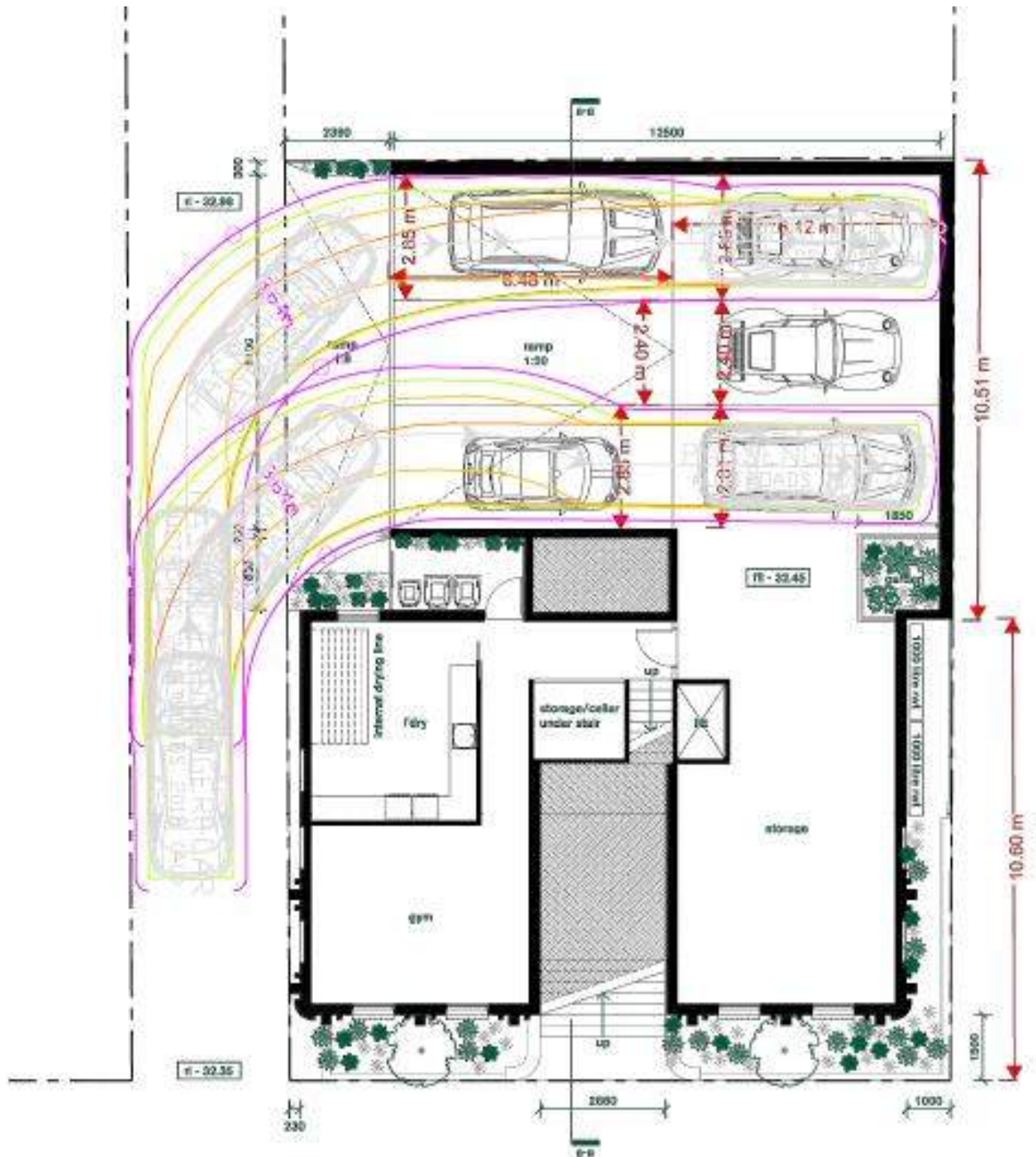
Figure 1: B99 vehicle manoeuvring within central space
