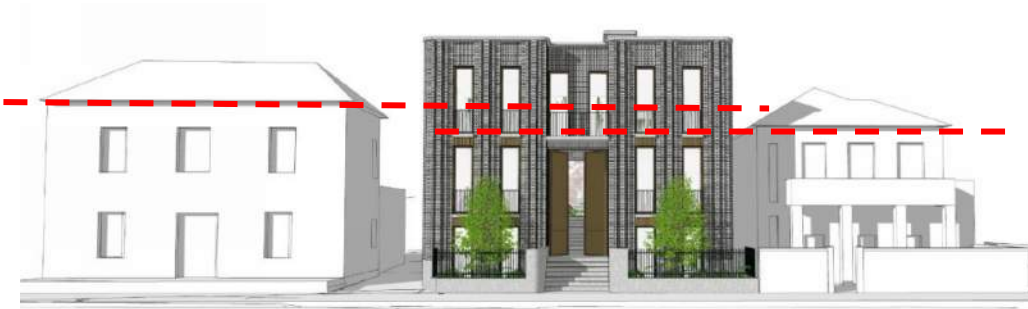
Figure 7: Base image from development application. Red horizontal lines inserted by URPS to illustrate height of facades of neighbouring buildings.
